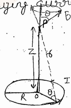
Here r is not in this plane while it is tilted by an angle  $\theta$
