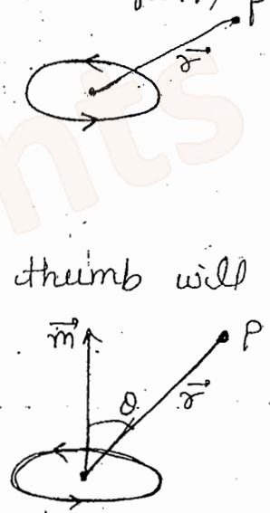
As Electric dipole mom. always directed along z-dir<sup>n</sup>. Here loop will be in x-y plane & mag. mom.  $\vec{m}$  is along z-axis & it will make  $\theta$  angle with  $\vec{r}$ ,
