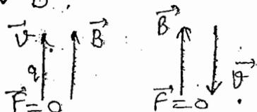
charged particle will move undeflected if  $v$  &  $B$  are parallel or antiparallel. [undeflected means straight line]
