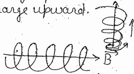
Ques 1:- An  $e^-$  enter in a uniform mag. field with magnitude  $0.3$  tesla, at an angle of  $45^\circ$  wrt to mag. field.
