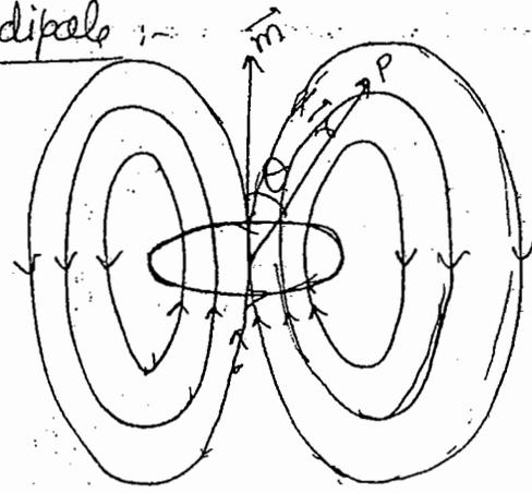
$$\begin{aligned} \vec{m} &= m \hat{z} \\ \text{dir}^n &\Rightarrow \vec{m} \times \hat{r} \\ \hat{z} \times \hat{r} &= \sin \theta \hat{\phi} \\ \text{i.e. dir}^n \text{ of } \vec{A} &= \hat{\phi} \end{aligned}$$
