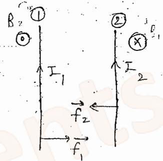
If current is in same dir<sup>n</sup> (for two wires) then force is attractive. This attraction is due to magnetic force.
