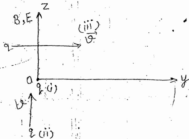
$v \perp$  to  $\vec{E}$  &  $\vec{B}$ ,  $v$  along  $y$  dir<sup>n</sup> &  $\vec{E}, \vec{B}$  along  $z$ -dir<sup>n</sup>  $\vec{E}$  push the charge particle in upward dir<sup>n</sup> &  $\vec{B}$  make the path helical in upward  $z$  dir<sup>n</sup>.
