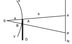
B is the new pole for finding itensity at P' half-period strips below B arer cut off by the obstacle only the uncovered half-period strips above B will be effective in producting illumination at P' as P' moves away from P, more no. of half period strips above B is also cut off & intensity gradually falls
