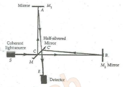
Measurement of wavelength: Using the Michelson interferometer, the wavelength of light from a monochromatic source can be determined. If  $M_1$  is moved forward or backward, circular fringes appear or disappear at the centre. The mirror is moved through a known distance d and the number N of fringes appearing or disappearing at the centre is counted. For one fringe to appear or disappear, the mirror must be moved through a distance of  $\lambda/2$ . Knowing this,
